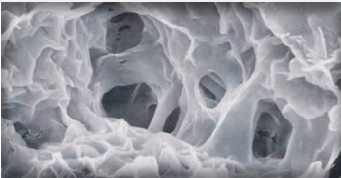
The absorbed product is encapsulated thanks to the particular structure of the fiber.
